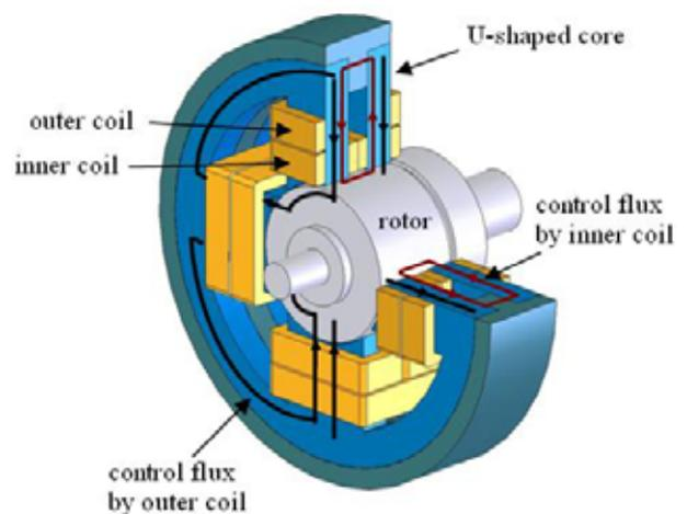
Fig. 1 Structure of the proposed AMB
