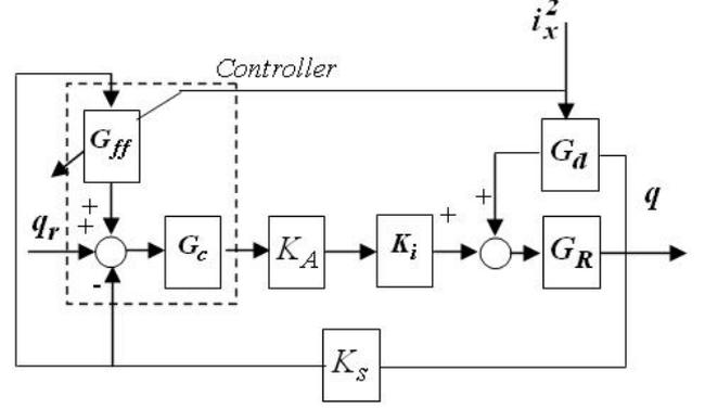
Fig. 4 Block diagram for radial controller with a feedforward loop
