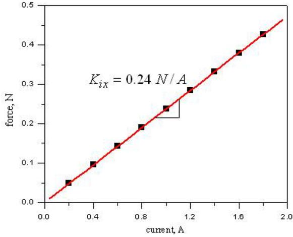
Fig. 5 FEM analysis results: axial control current versus force
