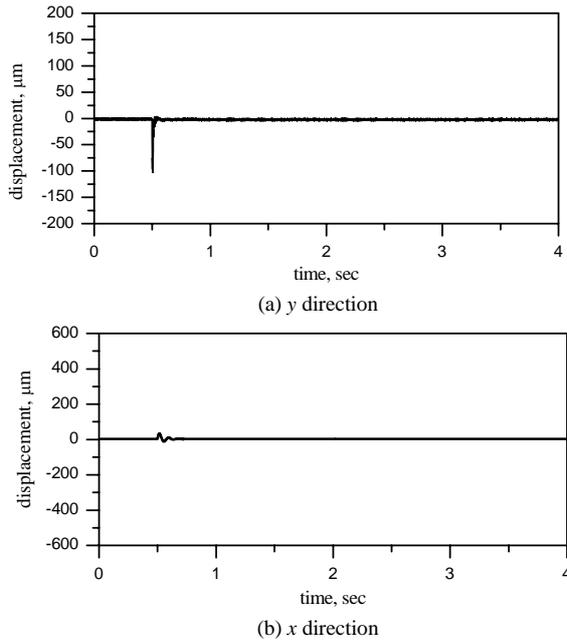
Fig. 8 Responses to y directional impulse under independent radial control
