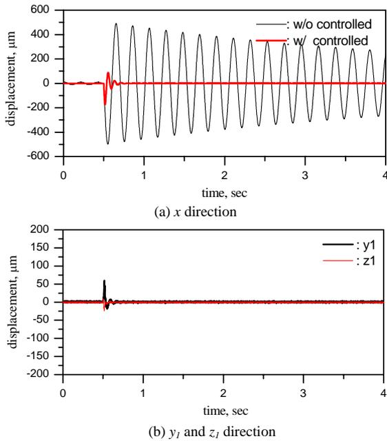
Fig. 9 Responses to x directional impulse under coupled radial control
