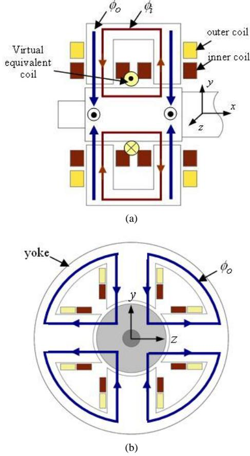
Fig. 2 Magnetic flux flow; (a) side view, (b) front view
