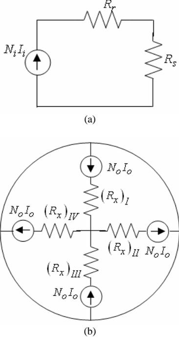
Fig. 3 Magnetic circuit models; (a) for inner coil, and (b) for outer coils
