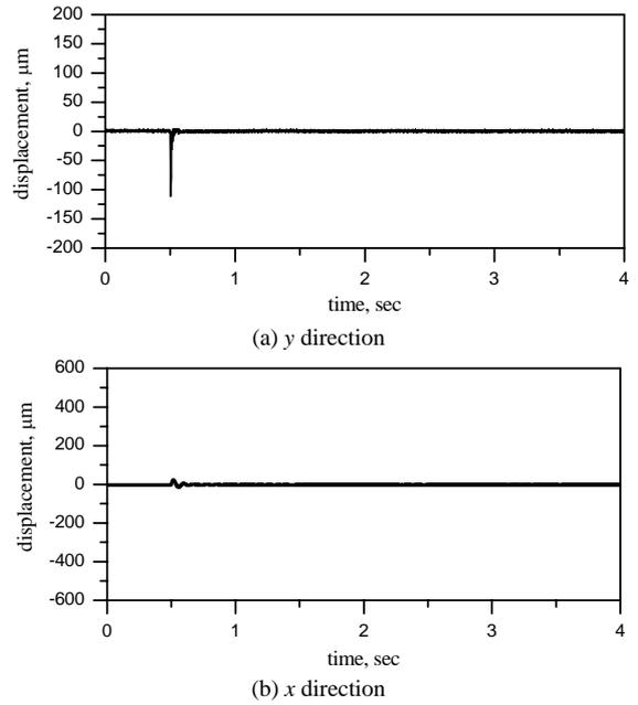
Fig.10 Responses to y directional impulse under coupled radial control
