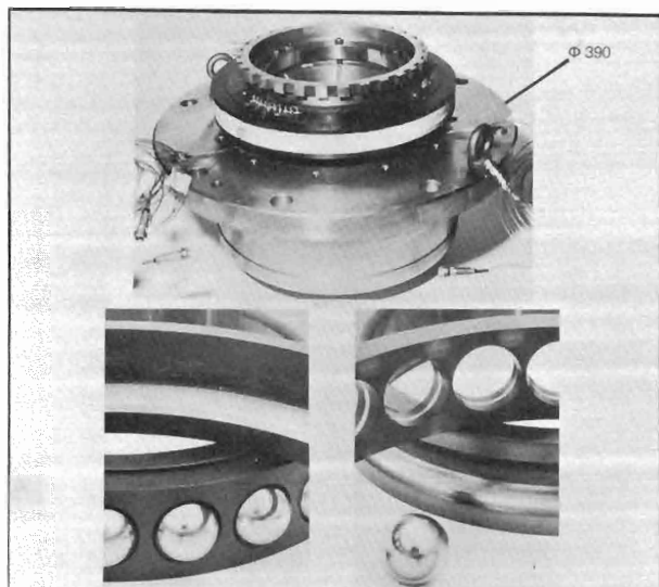
Complete Axial - Radial Retainer Bearing Unit and Ball Bearing Details
