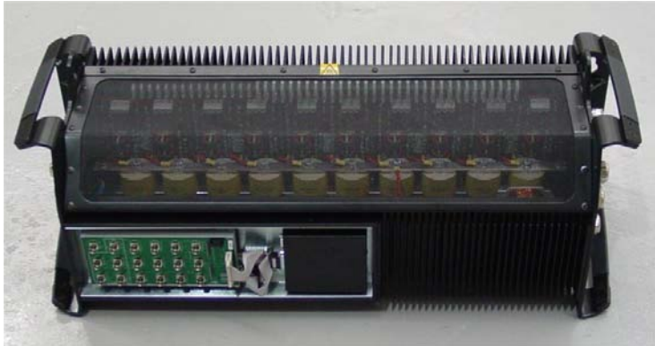
Figure 7 - Zephyr Controller (The control card of figure 3 is inside this unit)
