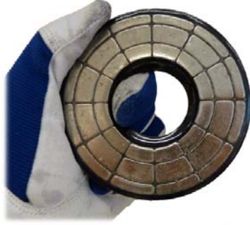
Figure 2: A segmented unit, which constitutes one half of the segmented Halbach bearing. The inner row is magnetized inwards, the middle row radially outwards and the outer row outwards.
