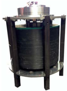
Figure 1: Photo of the flywheel prototype currently being finalized at Uppsala University.
