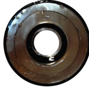
Figure 3: A ring-magnet unit, which constitutes one half of the Semi-segmented bearing, with magnetic fields directed inwards for the inner magnet. The opposite applies for the outer magnet.
