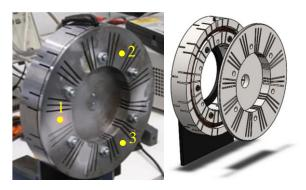
Fig. 2. Proof-of-concept electromechanical touchdown bearing mechanism in left and 3D model in right. Yellow points illustrate the location of eddy-current sensors.
