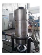
Fig. 1. High speed atomizer.
