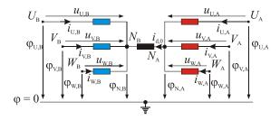
Fig. 3. Schematic representation of the six-phase winding in one half motor (Fig. 2) and definition of the currents and voltage potentials. The second winding in the second half motor is identical.
