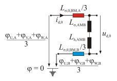
Fig. 5. Simplified inductive equivalent circuit of the zero-sequence component. The two half motors (BM: DE & NDE) are described by the two zero-sequence winding leakage inductances  $L_{\sigma,0,BM}$ . The axial magnetic bearing is described by a winding leakage inductance  $L_{\sigma,AMB}$  and a magnetizing inductance  $L_{h,AMB}$ .
