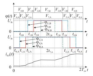
Fig. 4. Example of an asymmetrical pulse pattern for a six-phase system  $U_A$ ,  $V_A$ ,  $W_A$ ,  $U_B$ ,  $V_B$ ,  $W_B$  (e.g., DE BM) to produce a positive zero-voltage component and two equal active voltage space vectors  $(u_{\alpha,A}, u_{\beta,A})^T = (u_{\alpha,B}, u_{\beta,B})^T$ . The pulse width of the positive zero-voltage switching state  $V_7$  is larger in the winding A than in the winding B. Hence, the resulting zero-sequence current  $i_{d,0}$  increases.
